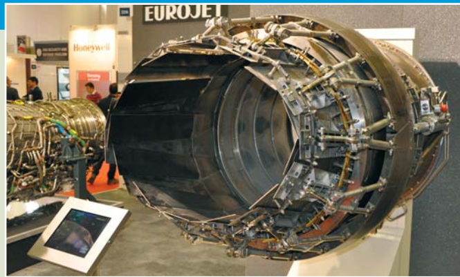
Eurojet also displayed the vectoring nozzle technology that is offered to Turkey.
