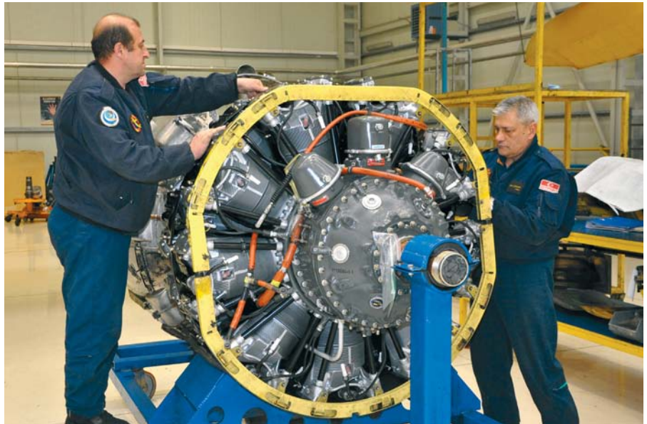
CL-215's internal combustion engine going through maintenance.
